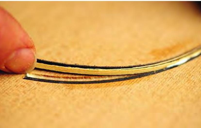
**9-27** Gluing four pieces in this channel
