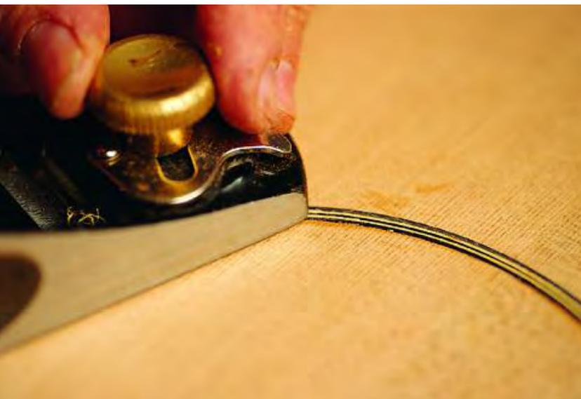
**9-28** Trimming flush with hand plane
